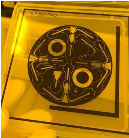
The Iridium Catalysed Electrolysis (ICE) CubeSat Thruster
